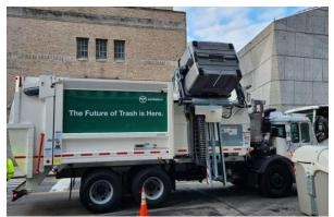
The Adams administration unveiled an all-new, automated, side-loading garbage truck — removing a major barrier to containerizing trash from high-density residential buildings. DSNY's 2023 "<u>Future of Trash</u>" report found that this type of truck is needed to service the stationary on-street containers that high-density buildings will use to containerize their trash.
